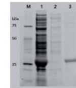
**Fig. 3** SDS-PAGE of two-step 6xHis-GFP purification; M: Marker; 1- lysate before purification; 2 - flow through; 3 - eluted 6xHis-GFP (27 kDa) after two-step purification
